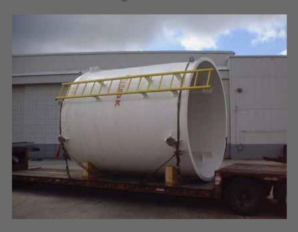
Oily waste storage: 8' diameter vessel.
