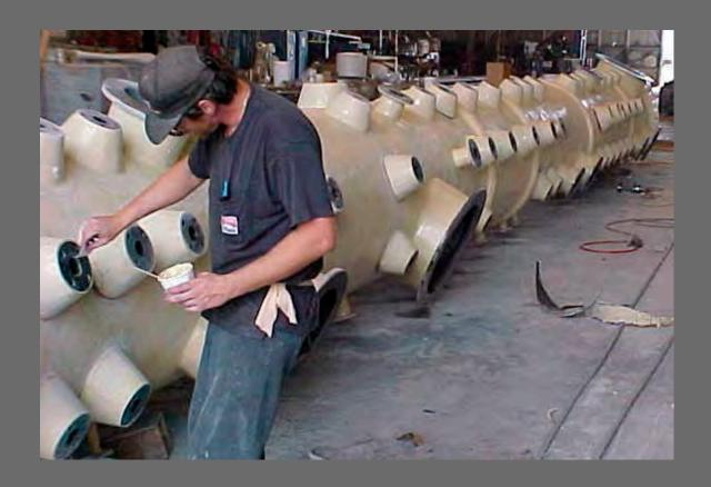
Pharmaceutical: Fume transfer ductwork (electrically conductive)
