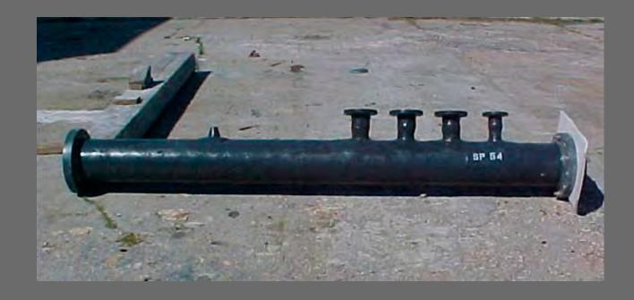
Chemical Plant: 10" diameter supply distribution header
