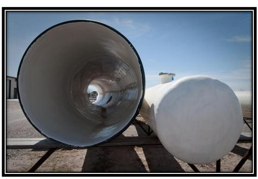
used. It is first coated with an appropriate release agent and the layup fabrication is started. The first material applied is normally a 10-mil layer of resin and special corrosion resistant glass called "C-glass". This reinforcing glass is in the form of a very thin veil or surfacing mat, similar in appearance to the "angel hair" used for Christmas decorations. This first 10-mil layer gives a high-resin, low glass content corrosion barrier.
